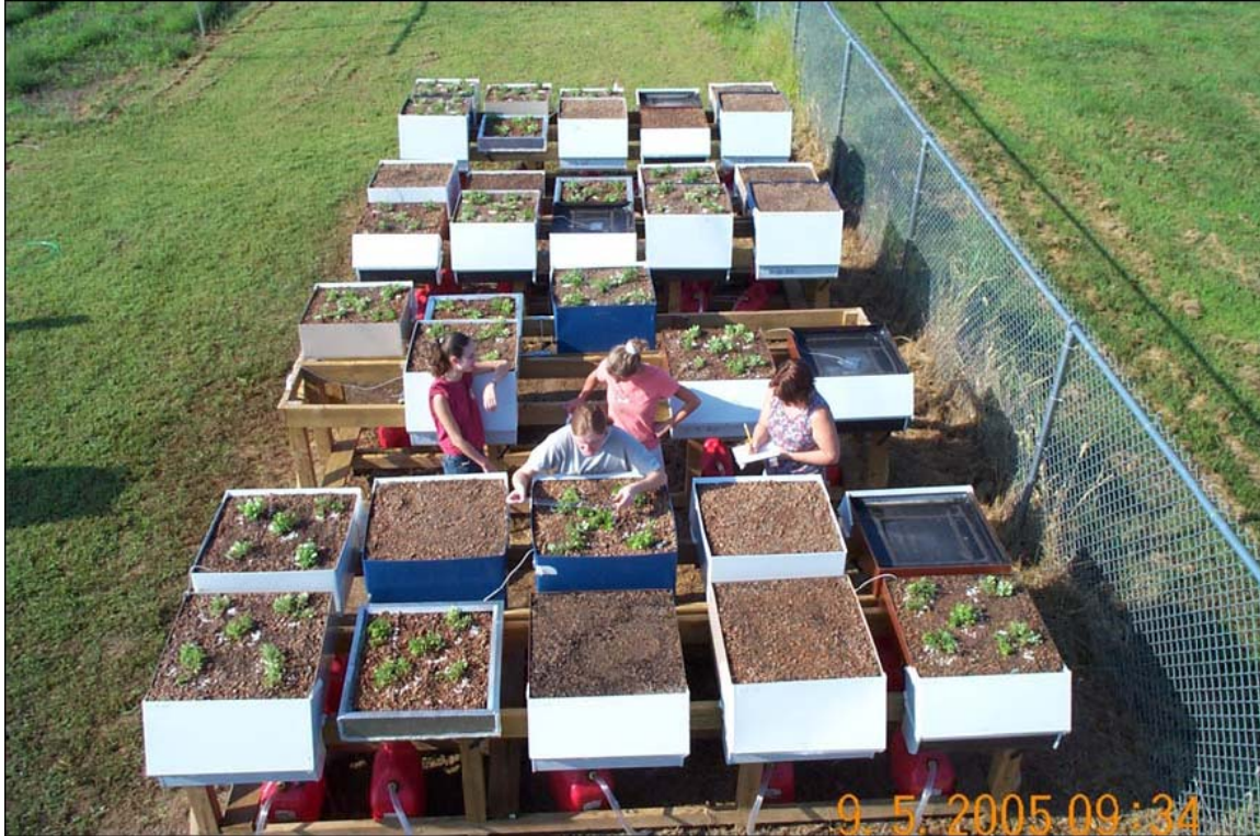
Figure 1. Green roof models with 5, 10, 15, and 20 cm growth medium depths at the Southern Illinois University Edwardsville Environmental Sciences Field Site.
