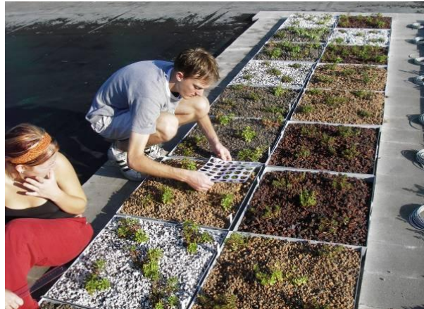
Figure 4: Undergraduate students recording roof coverage measurements with circle dot-grid. (These measurements were recorded twice a month during the early establishment period and once a month throughout the project).
