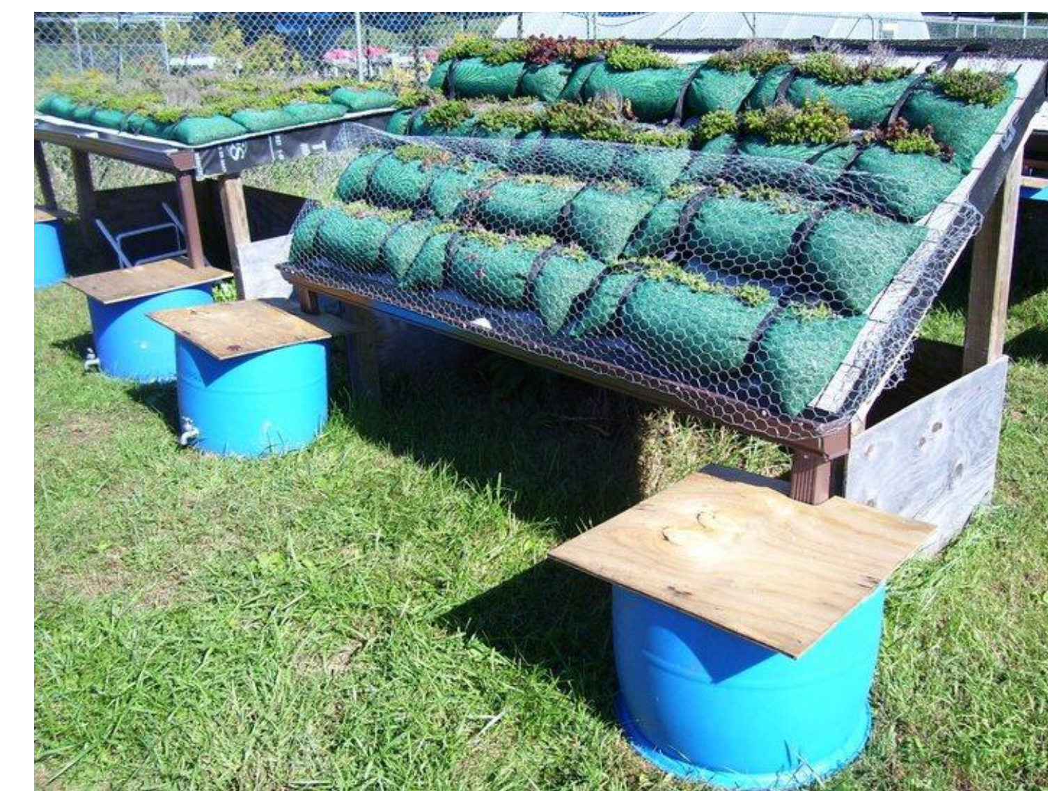
Figure 2. Residential green roof models at SIUE Environmental Science field site.
