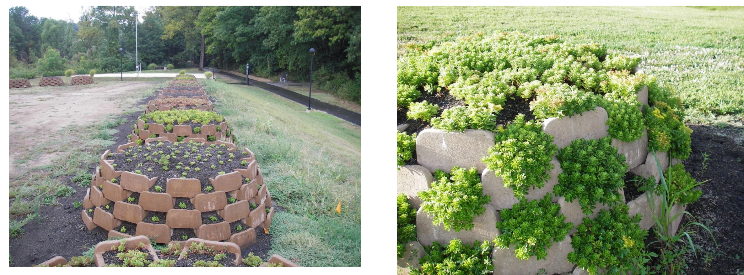
Figure 1. Eighteen circular living walls are being evaluated (left). Sedum species are planted in every pocket and on the top of each wall except the unplanted control wall (planted wall on right).
