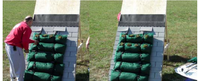
Figure 10. Prototype sloped green roof systems – testing to begin in 2007.
