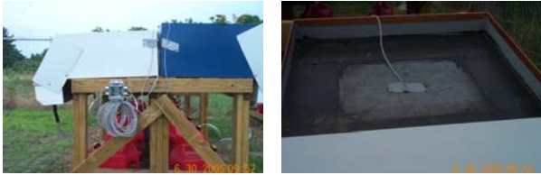
Figure 7. Built-in-place green roof models with thermal probes at the SIUE Environmental Sciences Field Site.
